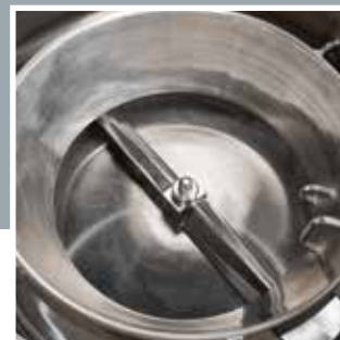
Kühlring Cooling cone
